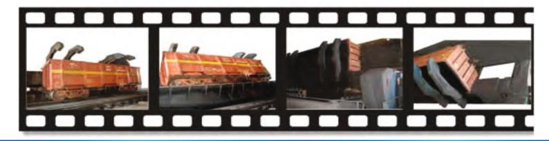
Capacity : Gross weight of loaded wagon 140 T (Max)
