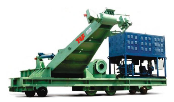
This Side Arm Charger with chain and sprocket design has haulage capacity of 15T. For 35T and above haulage capacity, Rack and pinion design Side Arm Charger is supplied. Our data given above is for Rack and pinion design. Haulage capacity, of Side Arm Charger is dependent on track layout on INHAUL side of Wagon Tippler
