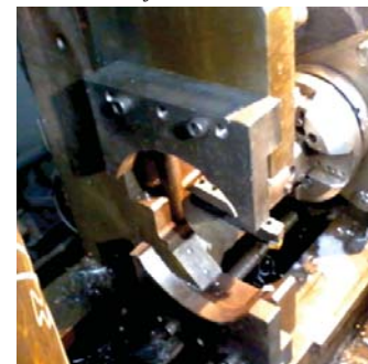
Additional jaw made and bolted to existing jaws on both sides of HB4 machine
