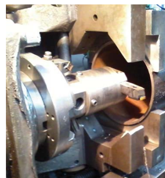
Modified 'boring bar & cutting tool' to 'reach' the job
